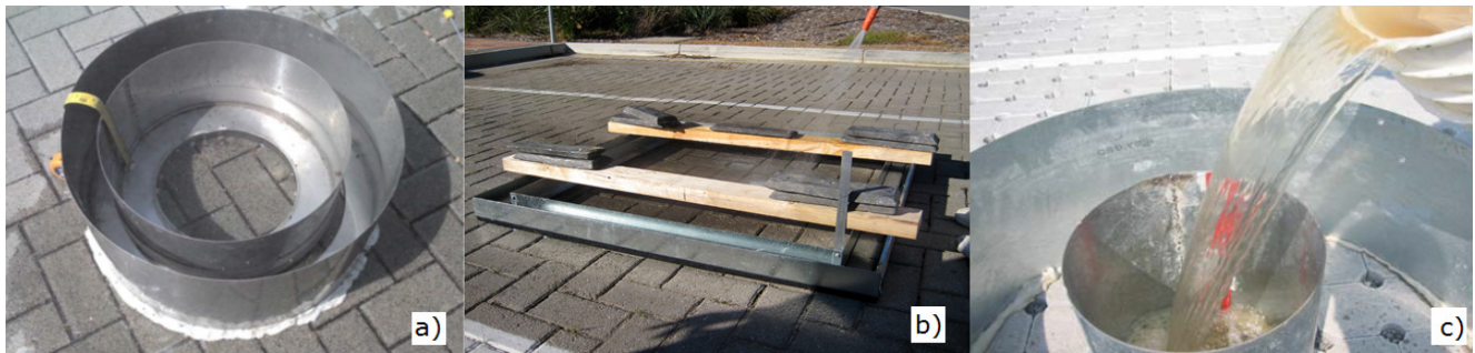
Figure 3. Modified ring infiltrometers used for permeable pavement testing: (a) double-ring infiltrometer tests (DRIT) [15]; (b) square, double-ring [13]; (c) single-ring surface inundation test [4].
