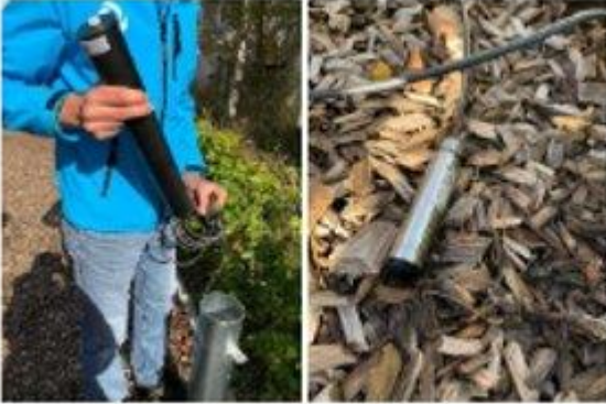
Figure 9 Photo of the housing (left) and the water level sensor (right)
